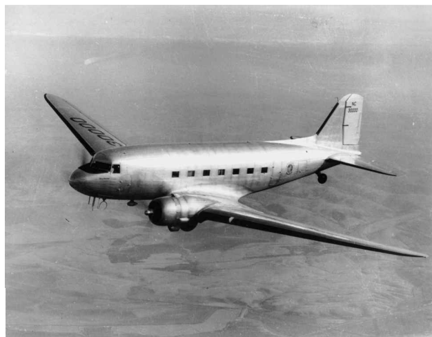
Fig. 9 Revolutionary all-metal Douglas DC-3 passenger airliner, introduced in 1935 (SI negative number A45861).
