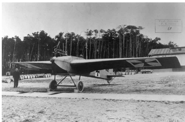
Fig. 12 Modern-looking, all-metal Junkers J-1 of 1915 (SI negative number A2493).
