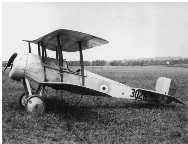
Fig. 2 Classic wire-braced, wood-and-fabric biplane that remained the standard structural design through the 1920s; this biplane is a World War I Bristol Scout (SI negative number 78-18721).
