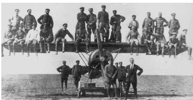
Fig. 5 Sleek 1918 Fokker D.VIII monoplane foreshadowed a coming standard with its thick-sectioned, plywood-sheeted, cantilevered single wing; Anthony Fokker, in front in necktie, humorously demonstrates the strength of the D.VIII wing design (SI negative number A2185).
