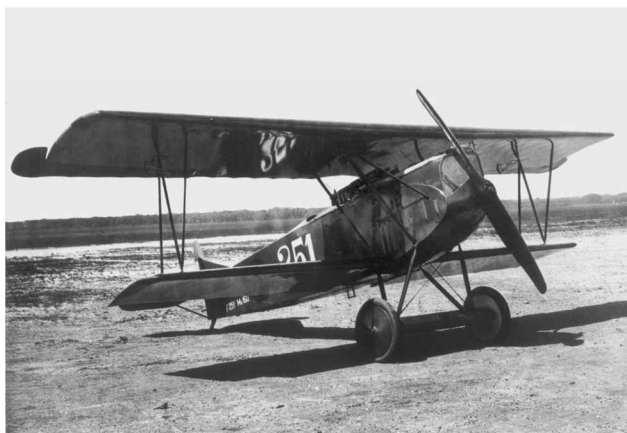
Fig. 4 Fokker D.VII had structural features similar to the Dr. I (SI negative number 94-7729).
