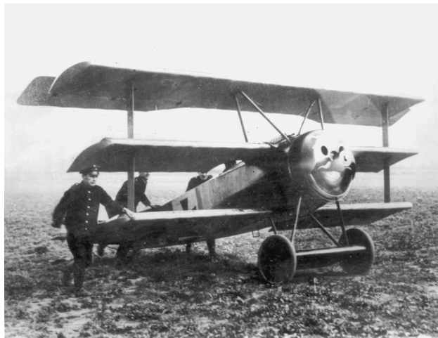
Fig. 3 Fokker Dr. I Triplane featured fabric-covered cantilevered wings with box spars; note the absence of wire bracing between the wings (SI negative number A9851-A).
