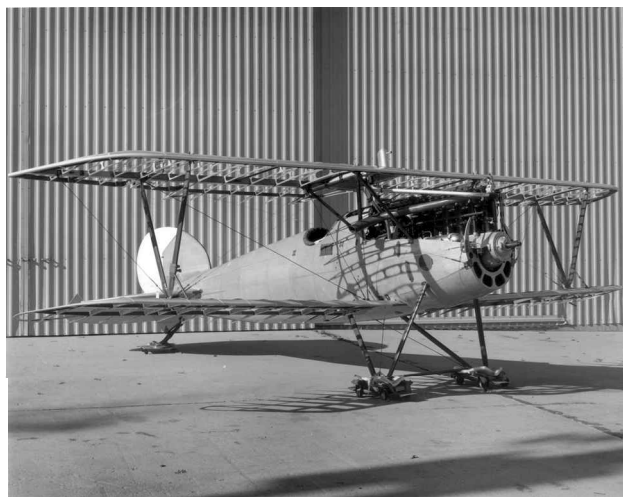
Fig. 6 Albatros fighter with fabric covering removed, showing its plywood monocoque fuselage (SI negative number 78-18979).
